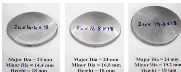
Fig. 6 Photograph showing billets after deformation using graphite + oil lubricant
