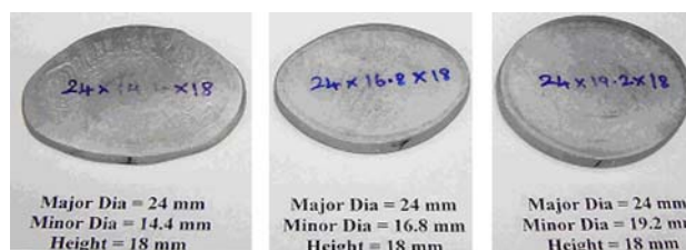
Fig. 5 Photograph showing billets after deformation using white grease lubricant
