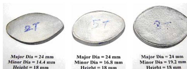
Fig. 4 Photograph showing billets after deformation using zinc sterrate lubricant
